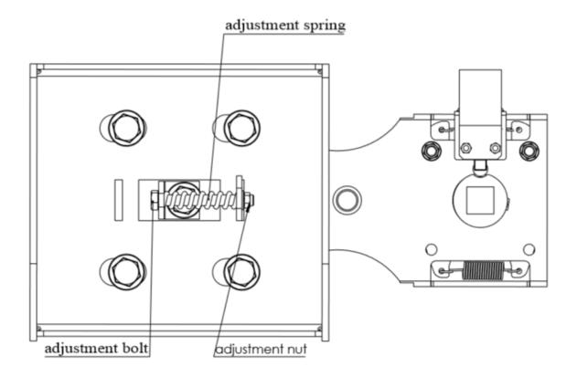
The brake block is adjusted with the adjustment bolt according to above dimensions. When system is actuated by pulling brake arm, easy working in system should be observed. Besides, both of blocks should be worked synchronously. This adjustment is very important to provide well force share during braking period. This adjustment is provided by tightening nut against adjustment bolt and by tightening contra nut adjustment is fastened.
