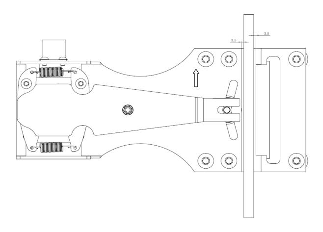
Distance between rail and roller must be 3 mm. Besides, distance between rail and both of brake shoes must be 3 mm, too. While these distances are being adjusted, the adjustments of brake shoes must not change.
